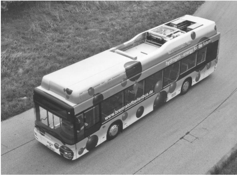
Figure 4.2 A fuel cell powered bus in use in Germany. Vehicles like this, used all day in cities, and refueling at one place, are particularly suited to being fuel cell powered (Reproduced by kind permission of MAN Nutzfahrzeuge AG.)
