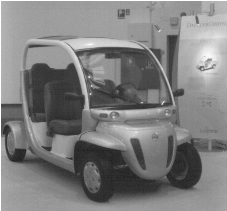
Figure 11.3 An example of the low speed vehicle (LSV) type of electric car
