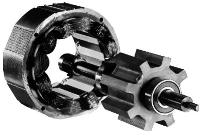
Figure 6.29 The rotor and stator from an SR motor (photograph reproduced by kind permission of SR Drives Ltd.)
