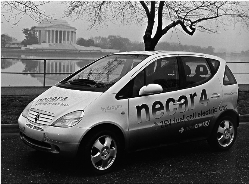
Figure 1.14 The Nekar 4 fuel cell car from 1999. This was the first fuel cell car to have a performance and range similar to IC engine vehicles. The top speed is 144kph, and the range 450km. The hydrogen fuel is stored as a liquid. (Photograph reproduced by kind permission of Ballard Power Systems.)
