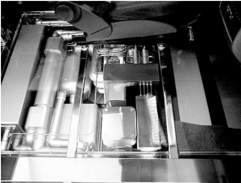
Figure 5.6 Packaging of the NeCar 5 methanol fuel processor
