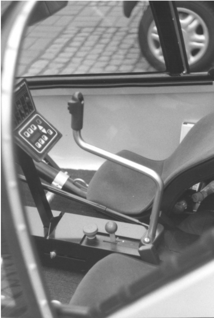
Figure 9.5 Stick controller fitted to a vehicle
