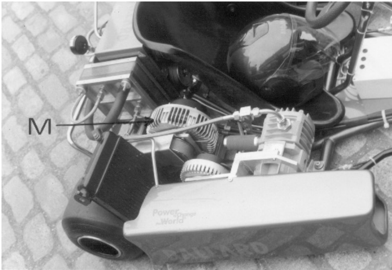
Figure 6.4 Small (10kW) DC ‘Lynch’ type DC motor, which is labelled M . This go-kart is fuel cell powered. The unit in front of the motor is the air pump, which is driven by its own motor, a smaller version of the traction motor
