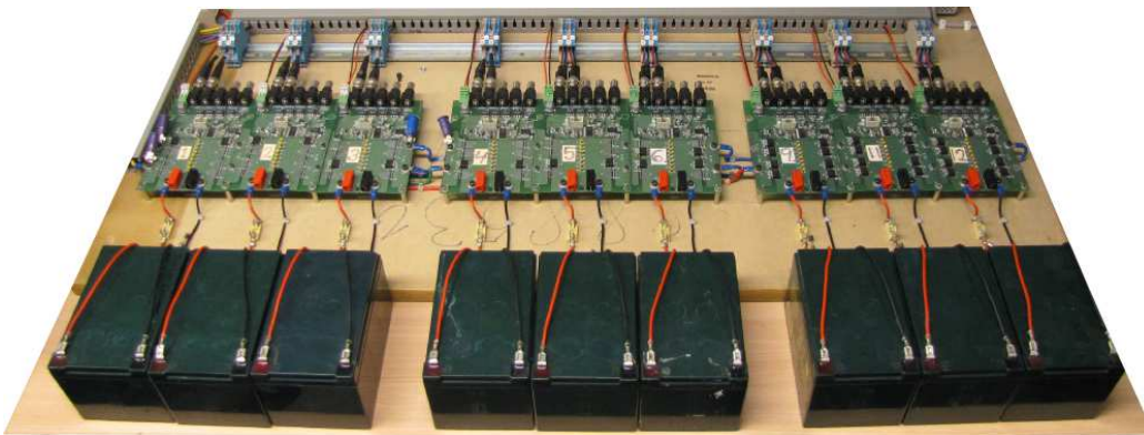
Figure 3.7: Laboratory setup of the 7-level multilevel inverter. The 3 phases consist of 3 levels each. The battery inputs are shown in the lower part of the picture, the outputs are on the left side of the groups and the common Y-connection point is shown on the right sides of the groups
