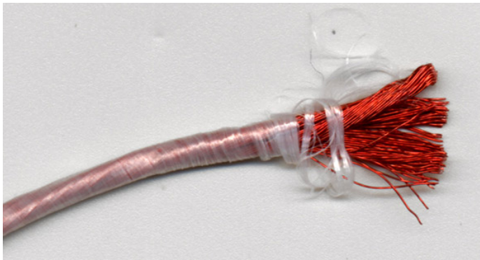
Fig. 2-4: Example of Litz wire
