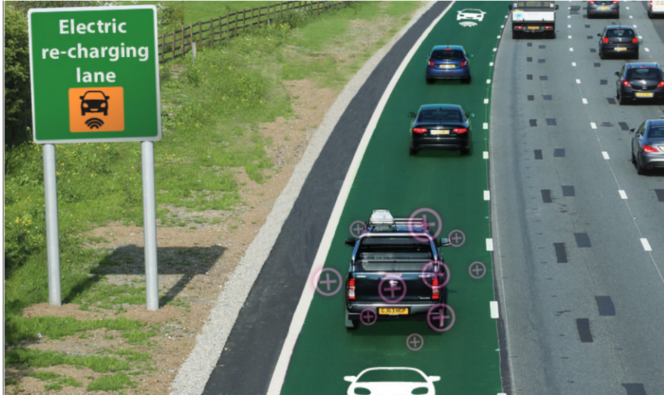
Figure 1.1: Illustration of dynamic charging of electric vehicles [8]. The EVs charge their batteries by moving along the left-most lane.
