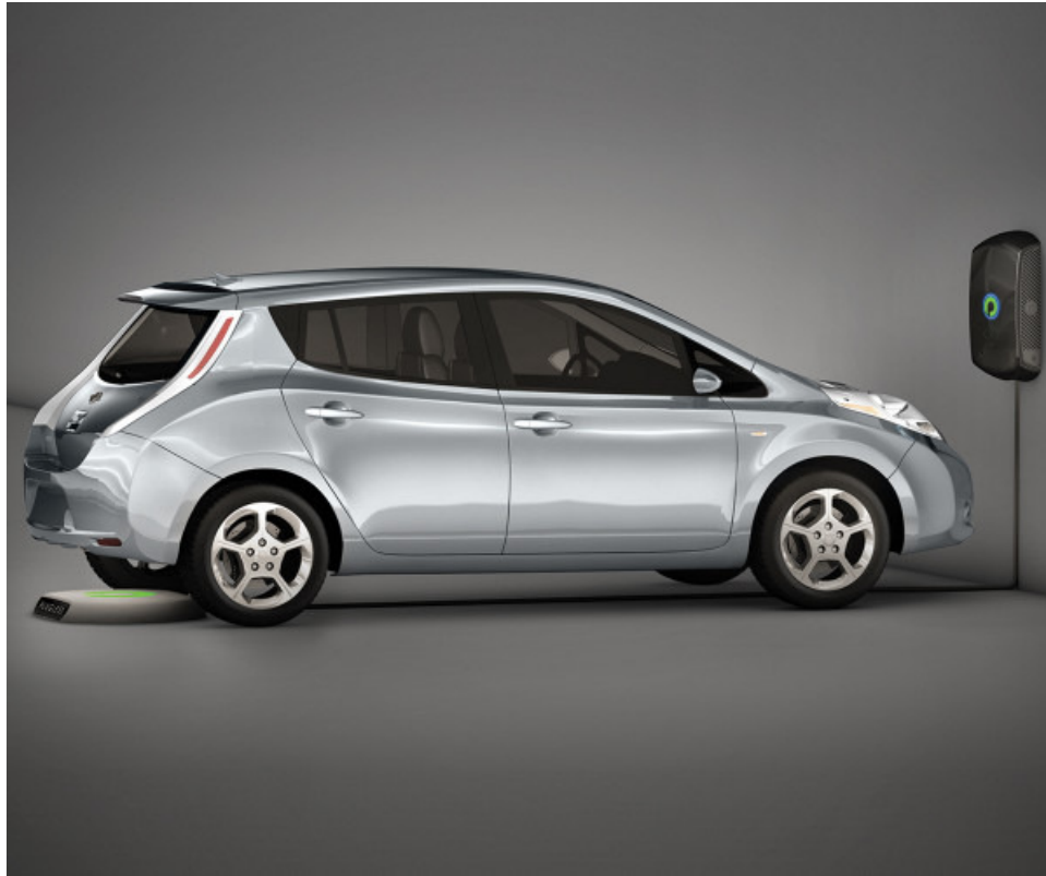
Figure 2.1: Plugless wireless charging system for Nissan Leaf showing the wireless charging pad and the wall-mount control panel [10].
