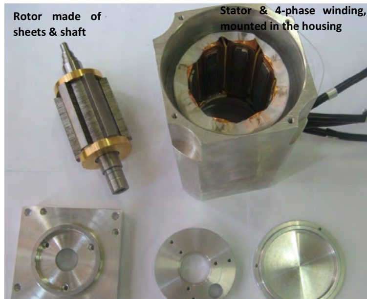
FIGURE 2-7. Photograph of the studied SRM, 8/6: stator, rotor and passive parts. [1]
