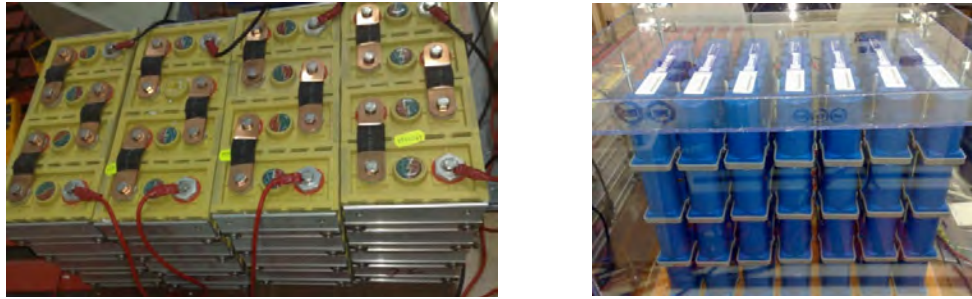
FIGURE 7-3. The battery (left) and UC (right) pack needed for the supply of the electric scooter.
