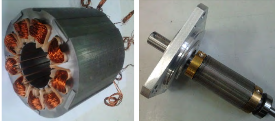
FIGURE 6-11. The stator with the coils around each tooth (left) and the rotor with the surface mounted magnets (right) of the constructed 9-phase-PMSM. [96]
