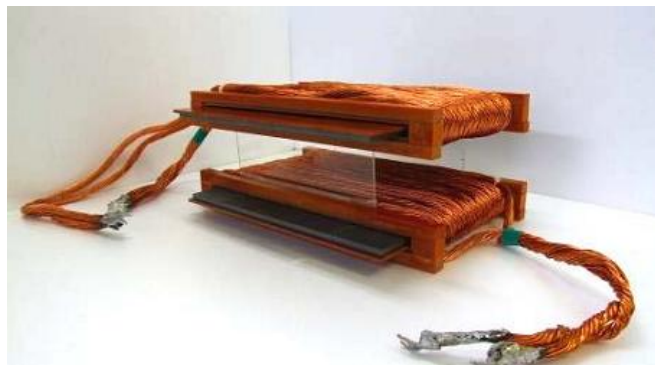
Fig. I.18. Photograph of the “FluxPipe”, showing the double-sided winding[96]
