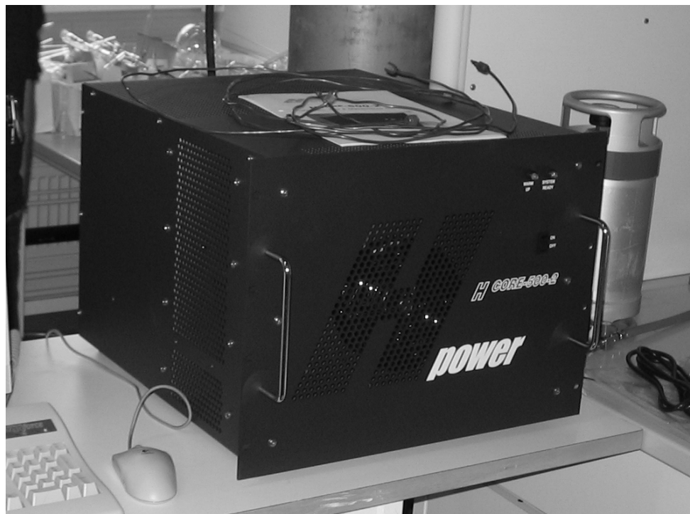
Figure 17. HCore-500-2 polymer electrolyte fuel cell. (photo: Pasi Paananen)
