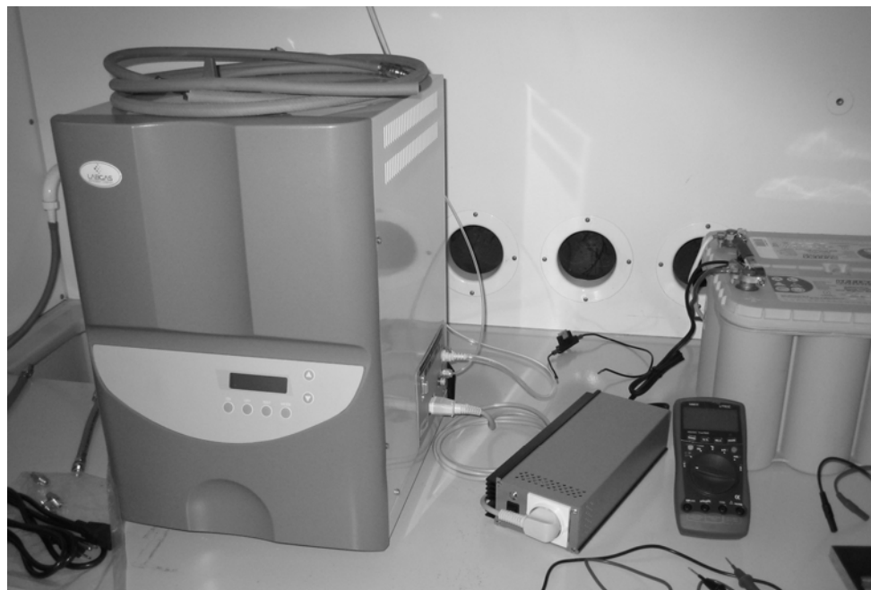
Figure 13. Electrolyser HG500, DC/AC inverter and the battery unit. (Photo: Pasi Paananen)
