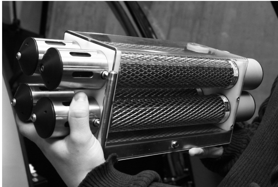
Figure 18. A fuel cell battery HC-400 (photo: RE program)
