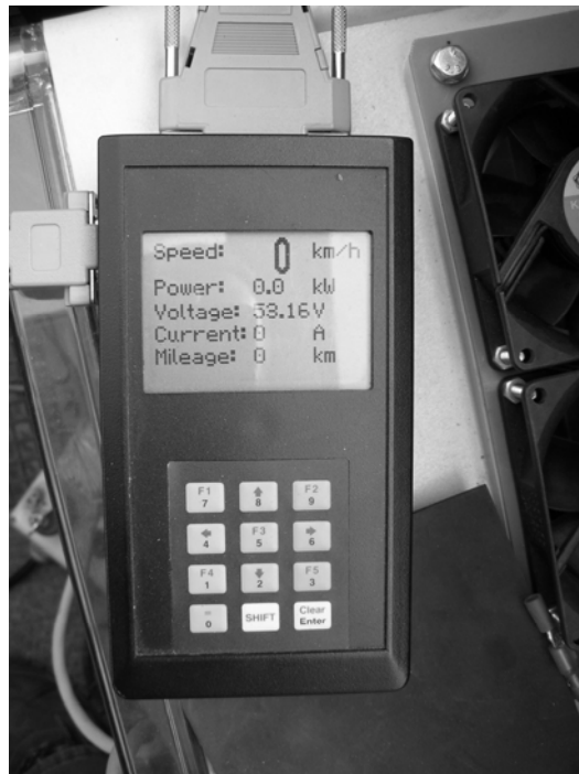
Figure 16. The external multimeter used as a data collection device during the test drive.
