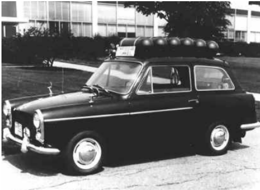
Figure 5. Hydrogen powered fuel cell passenger vehicle on public roads built by K. Kordesch in 1970 (Kordesch et al. 1999)
