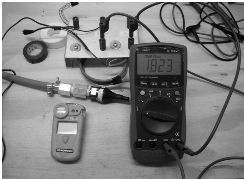
Figure 21. Some measuring equipment in the testing laboratory: portable leak detector, external pressure meter, plug board and a voltmeter.
