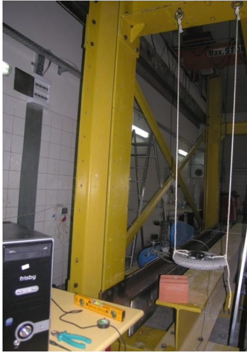
Figure 4.9 - Inertia Test Setup for Wheel
