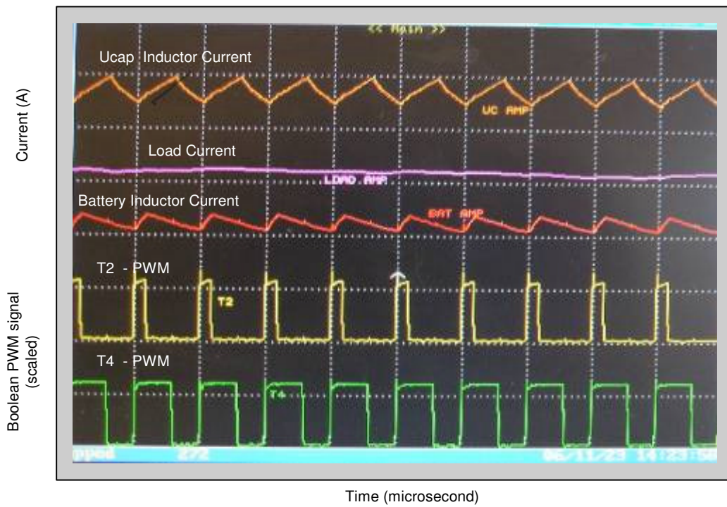
Figure 8.25 Measured PES parameters showing an ultracapacitor current increase
