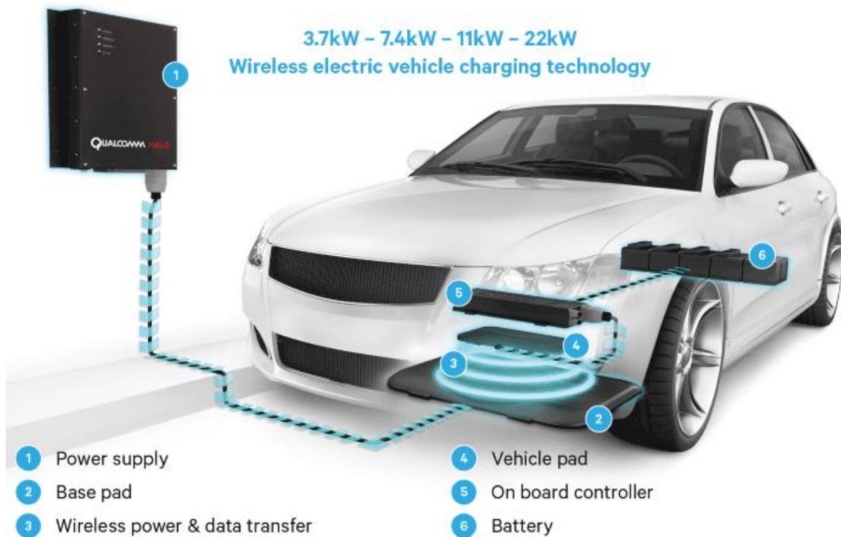
Static Wireless Charging System
