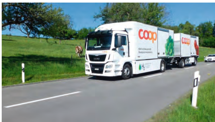
Figure 7: 34 t hydrogen fuel cell truck used by Coop (Source: www.esoro.ch )
