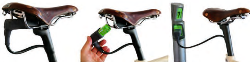
Figure 5: The IEC standardized socket which will be used around the world by all kinds of privately owned as well as by shared LEVs and bicycles to park them in accordance to public interests regulated by non-moving traffic management regulations (Source: EnergyBus)
