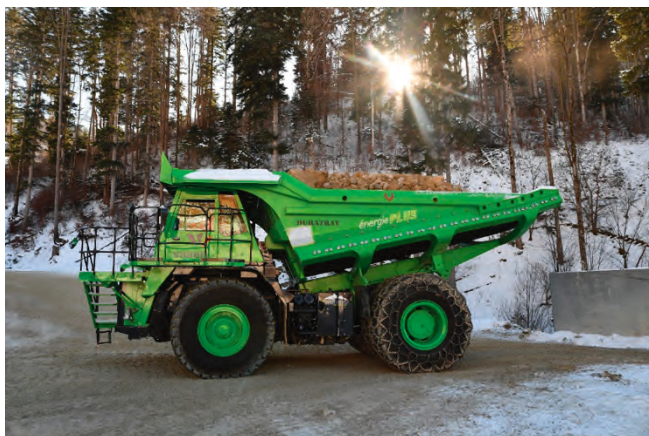
Figure 8: 110 t electric dumper truck at work in a quarry (Source: www.edumper.ch )
