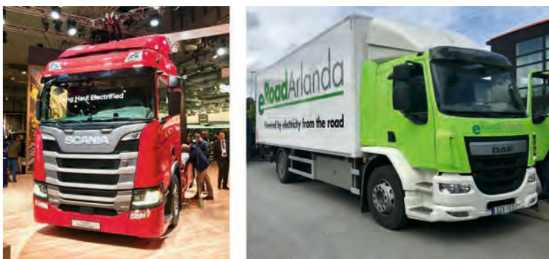
Figure 3: Scania plug-in hybrid trolley truck at the IAA Nfz fair 2018 (left) and electric converted DAF Truck tested in the eRoadArlanda (Sweden) project (right)
