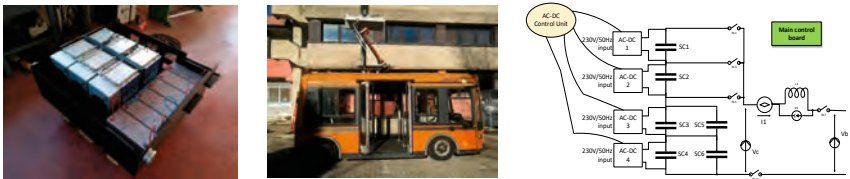
Figure 1: Storage system on board the bus (left), bus equipped with pantograph (middle) and electric schematic of the charging station (Source: ENEA)
