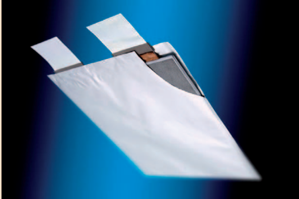
Inside of a high-power cell; the two electrodes can be seen at the top. (Fraunhofer ISIT)
