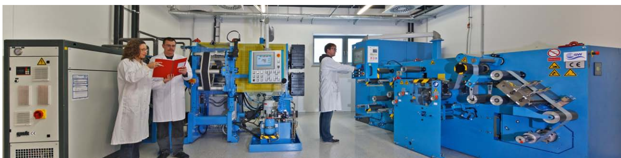
The calender, a system composed of several rollers, and the roller cutting machine for electrode production on the research production line in Ulm. (ZSW/M. Duckek)
