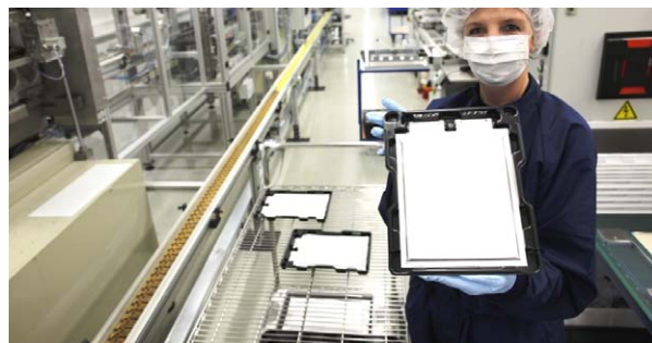
Dry room for battery cells (Li-Tec Battery GmbH)
