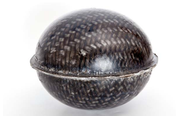
A component produced using the TwinOSheet method. (bielomatik Leuze GmbH + Co. KG)
