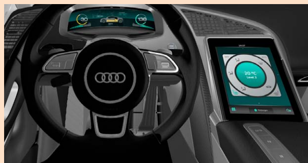
The cockpit is fitted with an iPad (on the right) that serves as the main control unit. (Audi AG)
