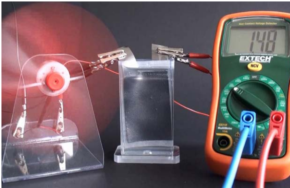
The battery experiment kit gives pupils a simple tool for making a lithium-ion battery. (Professor Marco Oetken and Martin Hasselman, Department of Chemistry, Freiburg University of Education)
