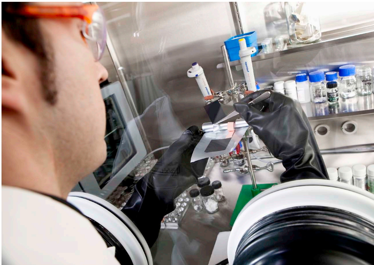
A chemistry lab technician assembling a lithium-ion test battery inside a glove box. The battery will be used to examine various new cathode materials. (BASF)
