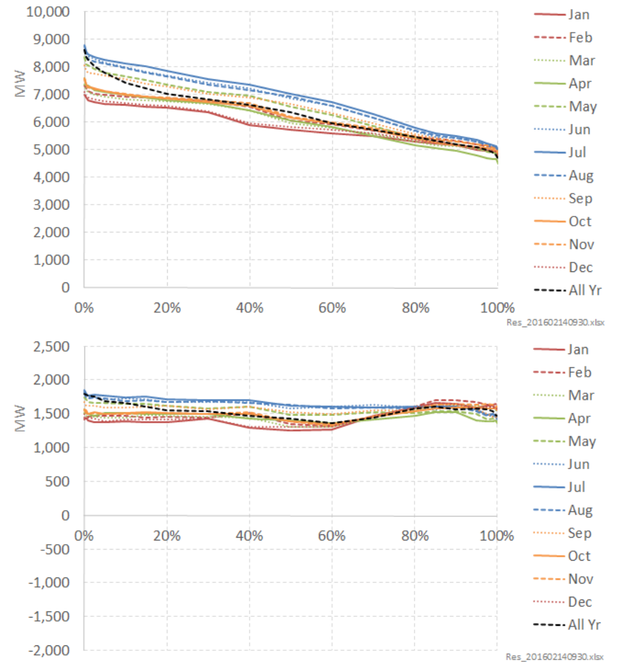
Figure 57: Projected 2036 demand duration curves (DCs) with high uptake of smart-charged EVs. A) Overall DC, and B) Change in DC over 20-year period
