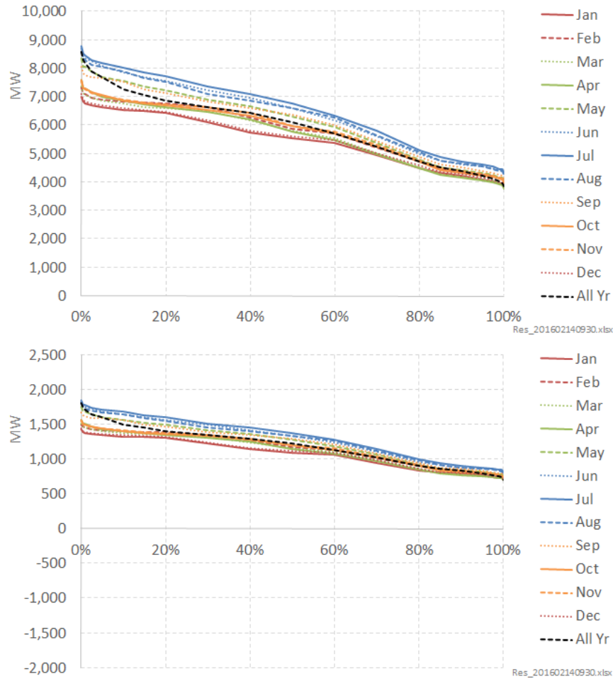
Figure 56: Projected 2036 demand duration curves (DCs) without EVs: A) Overall DC, and B) Change in DC over 20-year period
