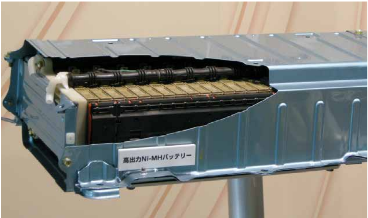
NiMH battery used in Toyota Prius
