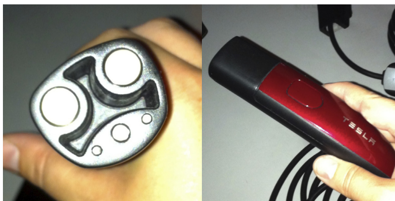
FIGURE D-4 The Tesla proprietary plug for DC fast charging is used for all Tesla DC fast chargers (Superchargers) now available in the United States. It is available only on the Tesla Model S. SOURCE: Gordon-Bloomfield (2011). Photo by Nikki Gordon-Bloomfield.
