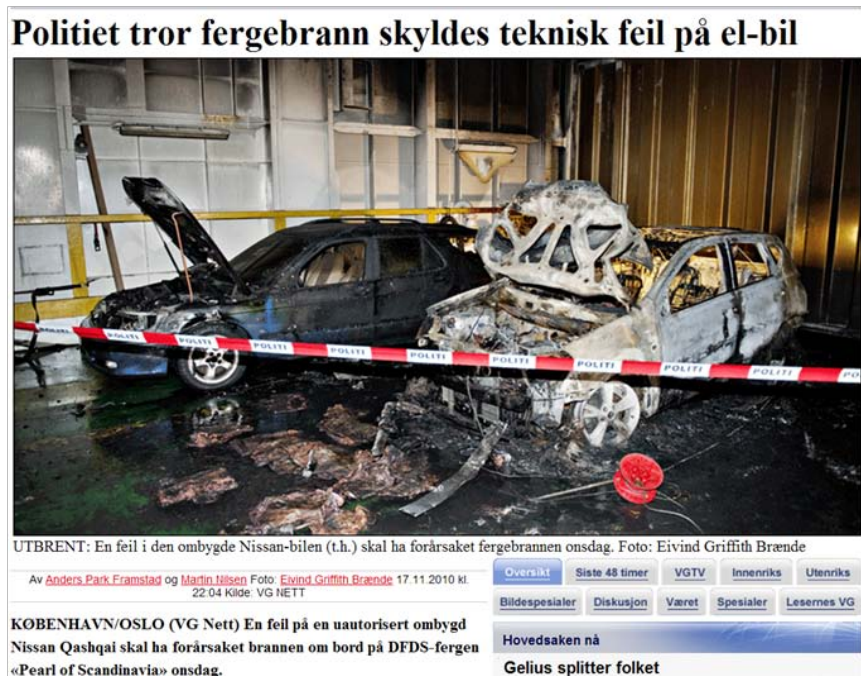
Figure 5: Fire with recharging of Electric cars on the DFDS ferry to Denmark. Source: www.vg.no .
