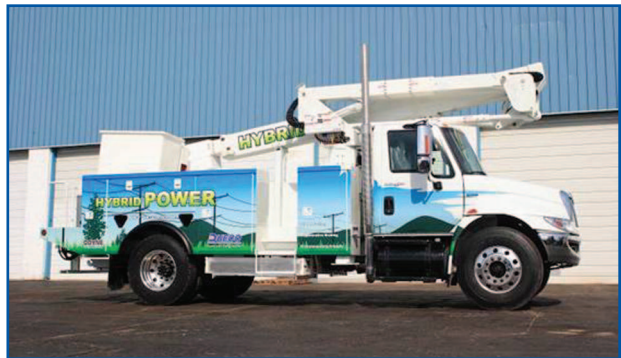
figure 1. Hybrid electric bucket truck for utility use. (Photo courtesy of Dueco.)
