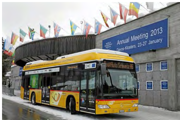
Fig. 26.2 One of two Mercedes-Benz Citaro FuelCELL hybrid vehicles provided by PostAuto Schweiz AG and tested during the World Economic Forum in Davos. (Image courtesy of Swiss Postauto.)
