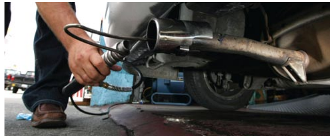
Measuring tailpipe emissions in a California Smog Inspection Station; the state has been a leader in clean air and pollution control for years.
