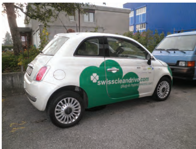
Fig. 27.7 SwissCleanDrive Fiat 500 converted to a plug-in hybrid car. (Photo: Solarcenter Muntwyler.)
