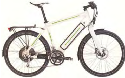
Fig. 27.12 The pedelec Stromer by Thömus, with a removable lithium-ion battery pack. (Photo courtesy of Thömus)
