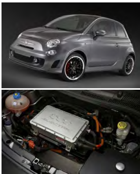
Fig. 22.2 FIAT 500 Electric with its electric drive. (Photo supplied by ENEA (from website)).
