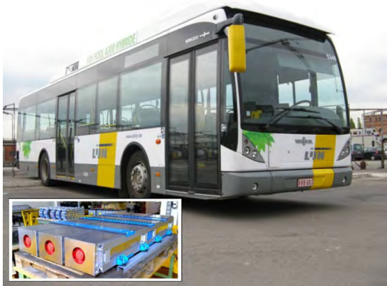
Fig. 15.3 Hybrid buses using ultracapacitors for brake-energy recovery (inset). (Photo courtesy of Van Hool.)
